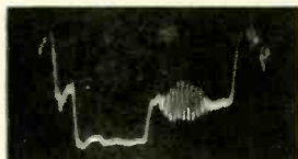
One horizontal sync pulse with its color burst.
