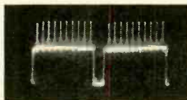
Square wave horizontal sync pulse with no back porch and poor dc coupling forces adjustments of brightness, contrast & fine tuning to obtain usable pattern.
