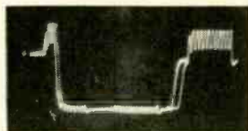
No back porch causes unstable color sync. Burst amplitude compression may permit sync on wrong color bar.
