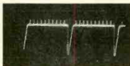
Complete absence of any back porch necessitates readjustment of brightness, contrast and fine tuning to obtain a usable pattern.
