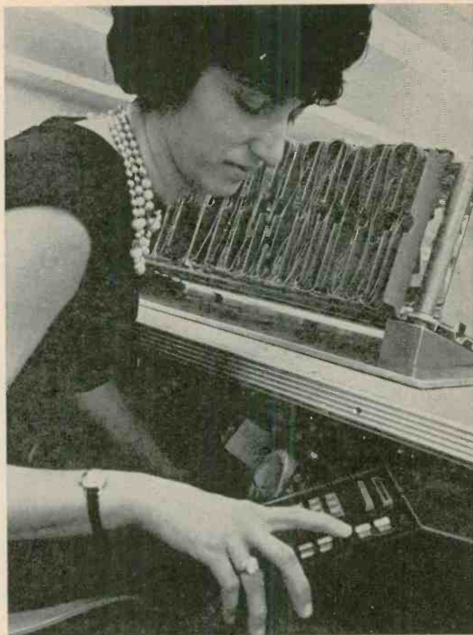
NO-TALK TELEPHONE MADE BY WESTERN ELECTRIC speeds filing of quality-control information. The instrument has new-style pushbuttons, but no handset. As worker tests an assembled product for quality, she "dials" data-storage department and "punches" her inspection results into a computer bank.
